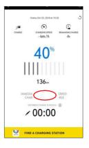
... you can program a starting time for charging the high-voltage battery.
